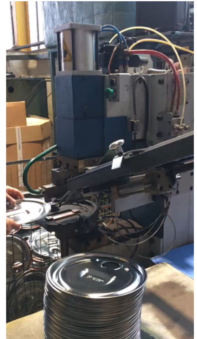
Figure 2: A spot welding machine used to weld handles on to metal lids
